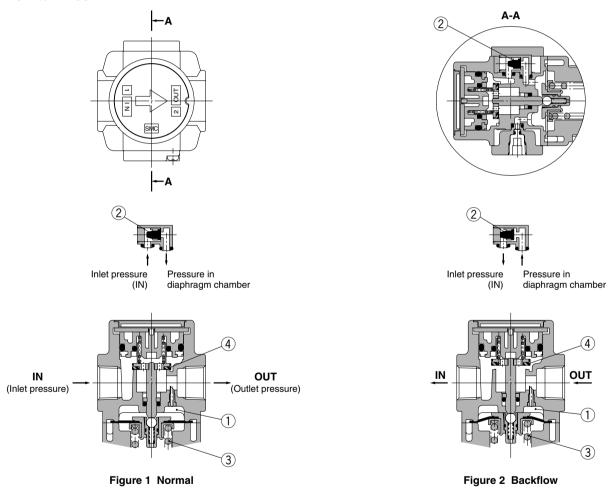
When the inlet pressure is higher than the regulating pressure, the check valve ② closes and operates as a normal regulator (Figure 1). When the inlet pressure is shut off and released, the check valve ② opens and the pressure in the diaphragm chamber ① is released into the inlet side (Figure 2).
