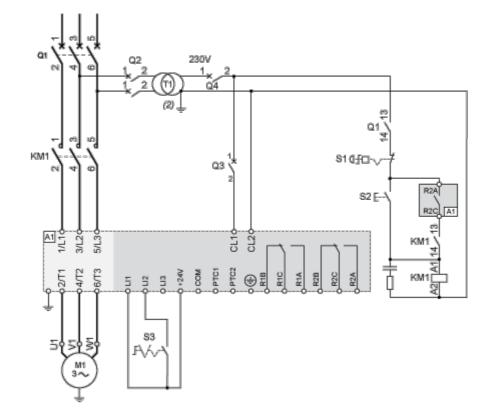
230 Vac control, logic Inputs (LI) 24 Vdc, 2-wire control, freewheel stop
