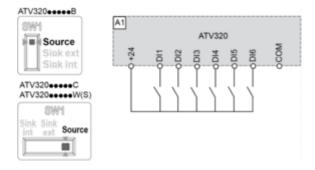
Switch SW1 set to "Source" position and use of an external power supply for the Dls.
