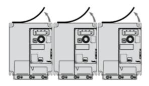
Mounting Type C: Individual, Ventilation Cover Removed
