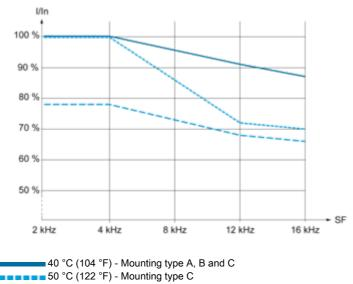
50 °C (122 °F) - Mounting type C 60 °C (140 °F) - Mounting type C In : Nominal Drive Current
