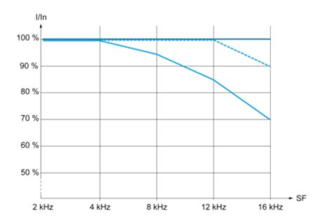
40 °C (104 °F) - Mounting type A, B and C 50 °C (122 °F) - Mounting type A, B and C 60 °C (140 °F) - Mounting type B and C
