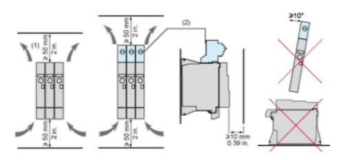
(1) Minimum value corresponding to thermal constraints.(2) Optional GV2 circuit-breaker
