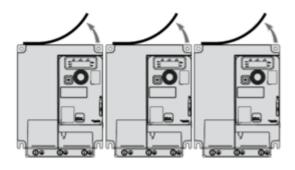
Mounting Type C: Individual, Ventilation Cover Removed
