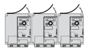
Mounting Type C: Individual, Ventilation Cover Removed
