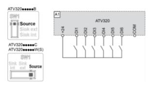
Switch SW1 set to "Source" position and use of an external power supply for the DIs.
