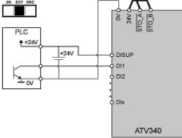
Digital Inputs: Internal supply Negative Logic, Sink, Asian Style
