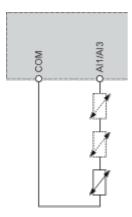
It is possible to connect either 1 or 3 sensors on terminals AI1/AI3.
