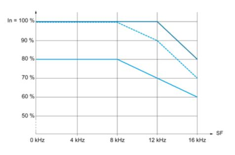
40 °C (104 °F) - Mounting type A, B and C 50 °C (122 °F) - Mounting type A, B and C 60 °C (140 °F) - Mounting type B and C In : Nominal Drive Current
