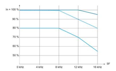
40 °C (104 °F) - Mounting type A, B and C 50 °C (122 °F) - Mounting type A, B and C 60 °C (140 °F) - Mounting type B and C
