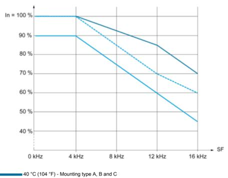
40 °C (104 °F) - Mounting type A, B and C 50 °C (122 °F) - Mounting type A, B and C 60 °C (140 °F) - Mounting type B and C In : Nominal Drive Current
