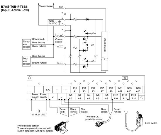
**Note:** 1. The wire colors have been changed in accordance with the revision of the Japanese Industrial Standards for photoelectric sensors and proximity sensors. The colors in parentheses refer to the old colors.
