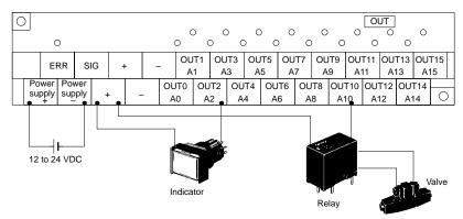
**Note:** Do not short-circuit terminals A and B, otherwise the internal element(s) of the B7A may be damaged.
