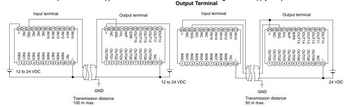
Note: A shielded cable with a thickness of 0.75 mm<sup>2</sup> min. must be used for signal transmission. It is recommended that the shield be grounded. The maximum transmission distance is 10 m if a VCTF wire with a thickness of 0.75 mm<sup>2</sup> is used instead of a shielded cable for the transmission path.
