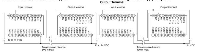
**Note:** A VCTF cable with a thickness of 0.75 mm<sup>2</sup> min. must be used for signal transmission.
