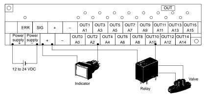
Note: Do not short-circuit terminals A and B , otherwise the internal element(s) of the B7A may be damaged. B7A-R6F11/-R6F16/-R6F31/-R6F36
