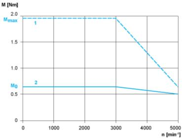
Servo Motor with LXM28AU02••• Servo Drive
