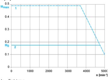
Servo Motor Without Shaft Sealing Ring and LXM28AUA5••• Servo Drive M [Nm]
