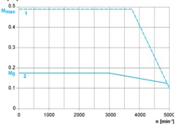
Servo Motor with shaft sealing ring and LXM28AUA5••• Servo Drive M [Nm]
