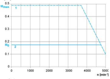
Servo Motor Without Shaft Sealing Ring and LXM28AUA5  $\bullet \bullet \bullet$  Servo Drive M [Nm]
