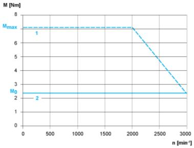
Servo Motor with LXM28AU04 ••• Servo Drive
