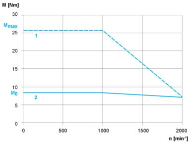
Servo Motor with LXM28AU10••• Servo Drive
