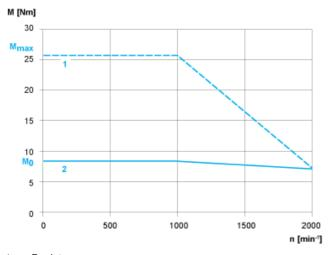
1: Peak torque2: Continuous torque
