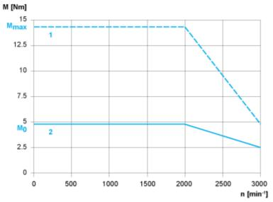
Servo Motor with LXM28AU10 ••• Servo Drive
