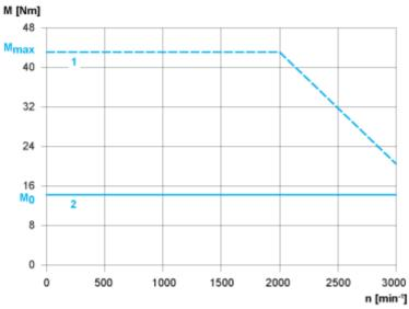
Servo Motor with LXM28AU30 ••• Servo Drive
