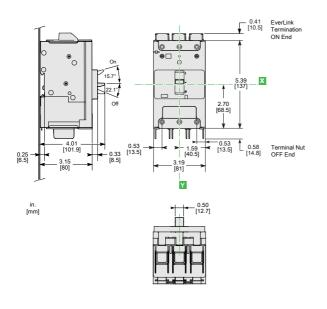
(M) TERMINATION OPTION - EverLink (ON end) / Terminal Nut (OFF end) ALL DIMENSIONS ARE APPROXIMATE. ALSO REFER TO CAD, TECHNICAL DRAWINGS, AND DOCUMENTATION
