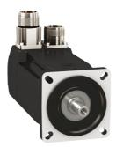
servo motor BMH, Lexium 32, 2.5Nm, 8000rpm, untapped shaft, without brake, IP54, 128 multiturn encoder, straight, 3 phases
