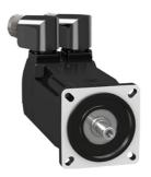
servo motor BMH, Lexium 32, 2.5Nm, 8000rpm, untapped shaft, without brake, IP54, 128 multiturn encoder, 3 phases
