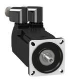
servo motor BMH, Lexium 32, 2.5Nm, 8000rpm, untapped shaft, with brake, IP65, IP67, 128bit encoder, 3 phases
