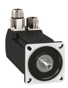
servo motor BMH, Lexium 32, 2.5Nm, 8000rpm, keyed shaft, without brake, IP65, IP67, 16bit encoder, straight, 3 phases
