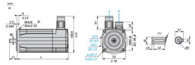
a: Power supply for servo motor brakeb: Power supply for servo motor encoder
