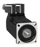
servo motor BMH, Lexium 32, 3.4Nm, 8000rpm, untapped shaft, with brake, IP54, 128 multiturn encoder
