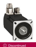
servo motor BMH, Lexium 32, 3.4Nm, 8000rpm, untapped shaft, without brake, IP54, 16 multiturn encoder, straight
