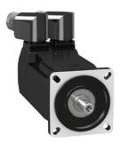
servo motor BMH, Lexium 32, 3.4Nm, 8000rpm, keyed shaft, without brake, IP54, 16 multiturn encoder
