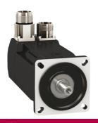
servo motor BMH, Lexium 32, 3.4Nm, 8000rpm, keyed shaft, with brake, IP54, 16 multiturn encoder, straight
