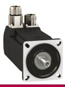
servo motor BMH, Lexium 32, 3.4Nm, 8000rpm, untapped shaft, without brake, IP65, IP67, 128 multiturn encoder, straight
