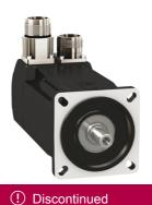
servo motor BMH, Lexium 32, 3.4Nm, 8000rpm, keyed shaft, without brake, IP65, IP67, 128 multiturn encoder, straight
