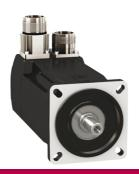
servo motor BMH, Lexium 32, 3.4Nm, 8000rpm, keyed shaft, without brake, IP65, IP67, 16bit encoder, straight
