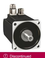
servo motor BMH, Lexium 32, 8.4Nm, 6000rpm, keyed shaft, with brake, IP65, IP67, 16 multiturn encoder, straight
