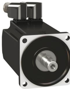
servo motor BMH, Lexium 32, 8.2Nm, 6000rpm, keyed shaft, with brake, IP65, IP67, 16 multturn encoder
