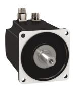
servo motor BMH, Lexium 32, 18.5Nm, 4000rpm, untapped shaft, without brake, IP65, IP67, 128 multiturn encoder, straight
