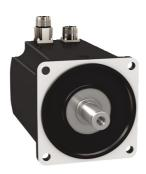
servo motor BMH, Lexium 32, 18.5Nm, 4000rpm, untapped shaft, without brake, IP65, IP67, 16bit encoder, straight
