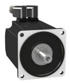
servo motor BMH, Lexium 32, 18.5Nm, 4000rpm, untapped shaft, without brake, IP65, IP67, 16bit encoder
