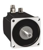
servo motor BMH, Lexium 32, 18.5Nm, 4000rpm, keyed shaft, with brake, IP65, IP67, 128 multiturn encoder, straight
