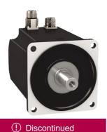
servo motor BMH, Lexium 32, 24Nm, 4000rpm, untapped shaft, with brake, IP54, 128 multiturn encoder, straight, 3 phases
