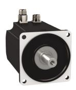
servo motor BMH, Lexium 32, 10.3Nm, 4000rpm, keyed shaft, without brake, IP54, 128bit encoder, straight
