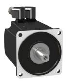
servo motor BMH, Lexium 32, 24Nm, 4000rpm, keyed shaft, with brake, IP65, IP67, 16bit encoder, 3 phases
