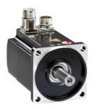
servo motor BMH, Lexium 32, 34.4Nm, 3800rpm, untapped shaft, with brake, IP54, 128bit encoder, straight
