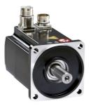
servo motor BMH, Lexium 32, 34.4Nm, 3800rpm, keyed shaft, without brake, IP54, 16bit encoder, straight
