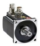
servo motor BMH, Lexium 32, 34.4Nm, 3800rpm, untapped shaft, without brake, IP65, IP67, 128bit encoder, straight
