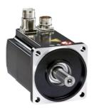
servo motor BMH, Lexium 32, 34.4Nm, 3800rpm, untapped shaft, without brake, IP65, IP67, 16 multiturn encoder
